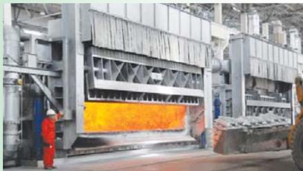
• Tilt smelting furnace powered by LNG
